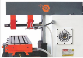
Robust Designed Headstock with Rigid Overarm, Arbor & Supports
